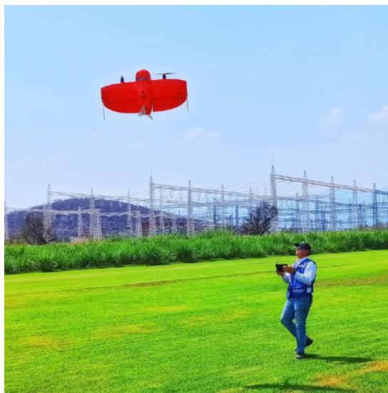
Photo 8: Conducting photogrammetric drone flights to generate orthophotos, digital twins, and cartographic products, aimed at emergency response following Hurricane Otis, 2024.
