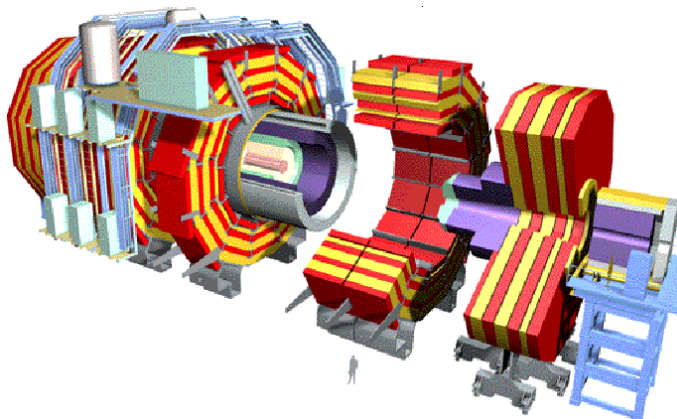
Figure 1 CMS – diameter : 14.60 m, length : 21.60 m, weight : 14600 tons.
