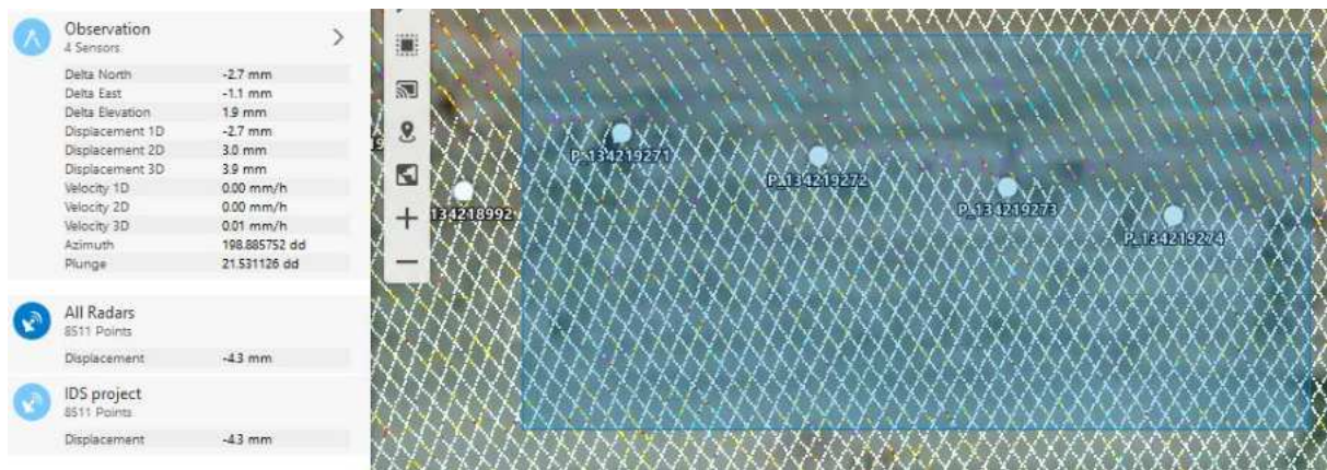
Figure 8 Cross-analysis of prism and radar monitoring data
