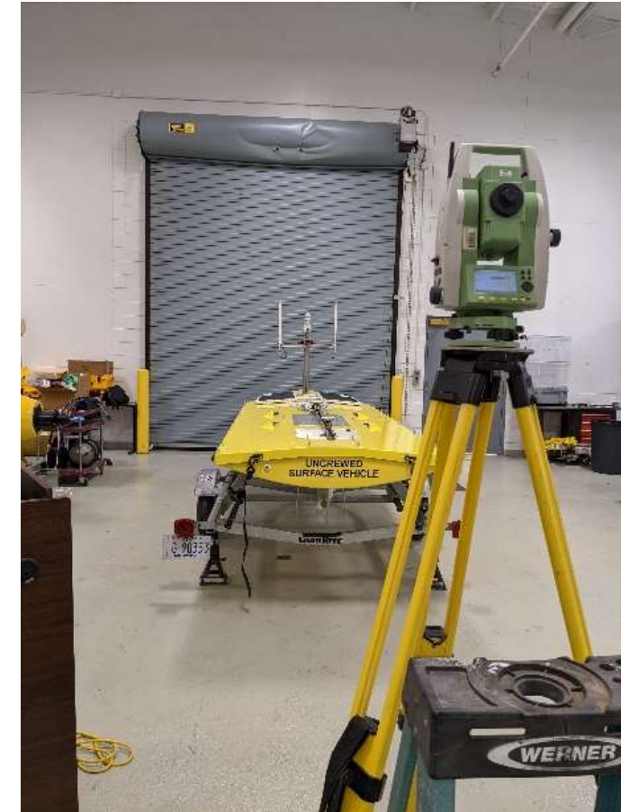
Experiment #2: Offsets/ lever-arms measurement with total station
