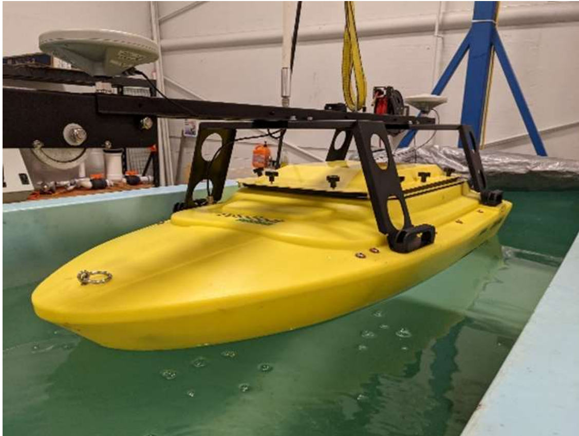
Experiment #1: Offsets/lever-arm measurement with tape
