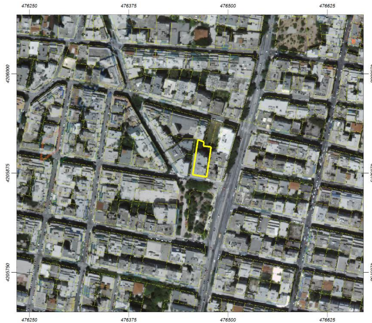
Figure 6: Cadastral Diagram excerpt of no-normal urban plot shape, Athens Municipality, Attica Prefecture (Source: Hellenic Cadastre web map, accessed 10/03/2023)
