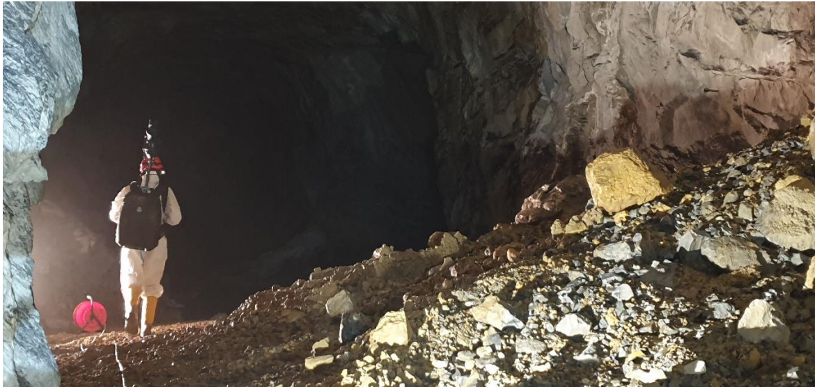
Figure 6: Mapping the underground mine by HERON MS TWIN COLOR
