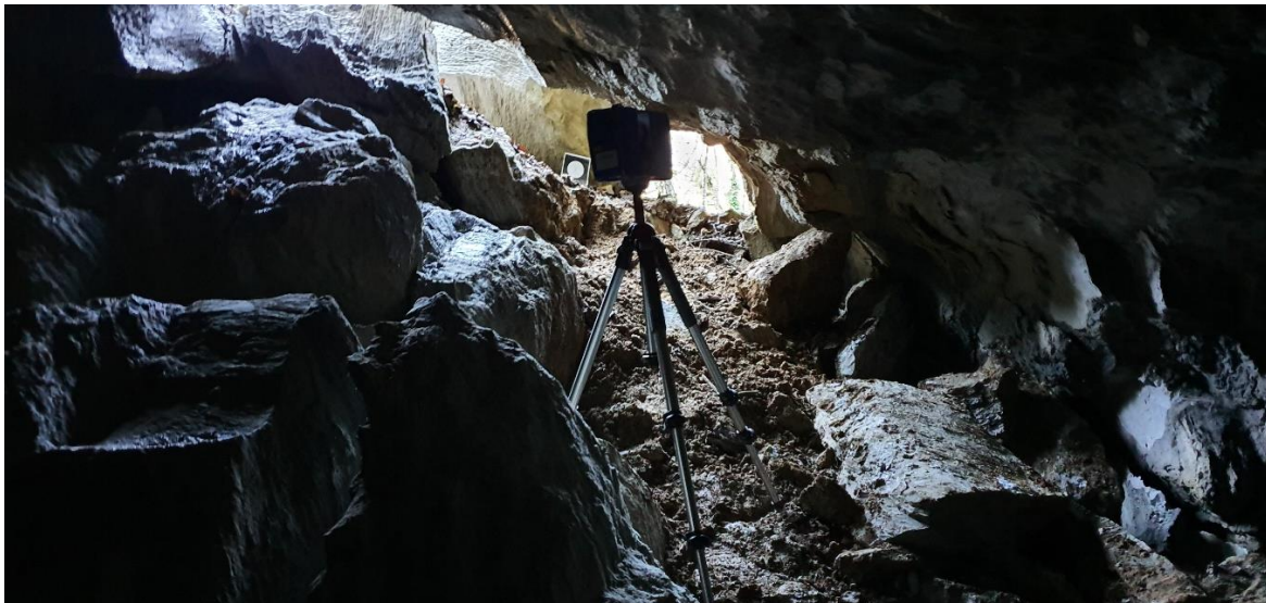
Figure 7: The scanning phase to connect with TLS the underground mine with the outdoor
