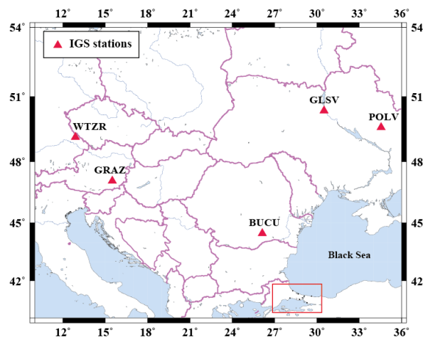
Figure 2. IGS stations used as a reference for the relative point positioning (red rectangle represents the study area)
