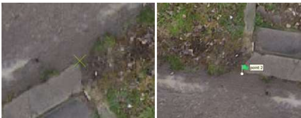
Figure 9: Measurement of point position on orthomosaic (left) and image (right)
