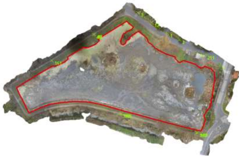
Figure 8: Configuration of the check points used for the precision evaluation (green) and the new cadastral boundary extracted from the orthomosaic (red)
