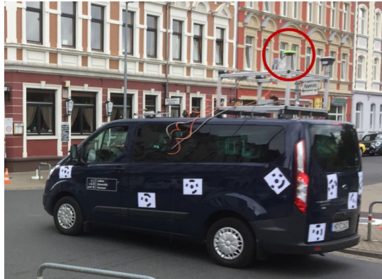
Figure 3: IfE measurement van during the kinematic experiment. The antenna in use is circled in red.
