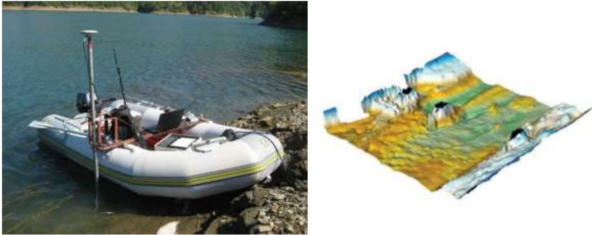
Figure 3. Boat equipped with echo sounder and GPS device (left) and 3D view of the river bottom measured with multi beam echo sounder (right) (Source: IJČ, 2018)
