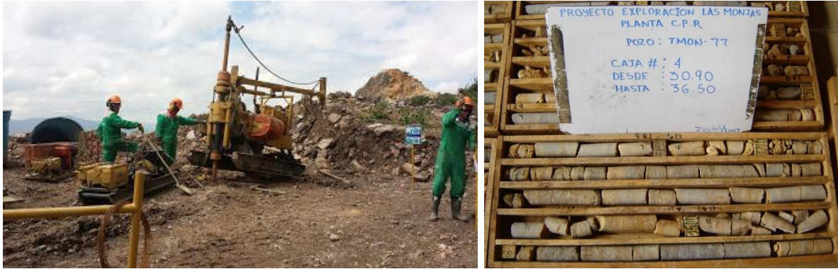
Image No. 3 drill drilling with core recovery, next to the cores arranged in the box with their corresponding interval ready for the Logueo. Source: Argos
