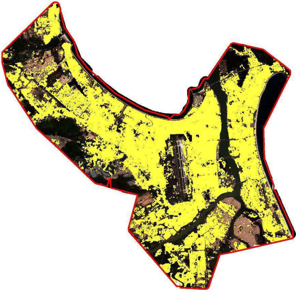
Figure 4 Rooftop in the AOI in Da Nang city were detected by the O-O method
