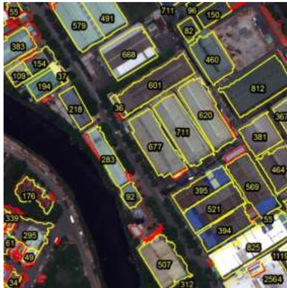
Figure 7 Examples of total yearly PV energy produced by HCMC rooftops in MWh
