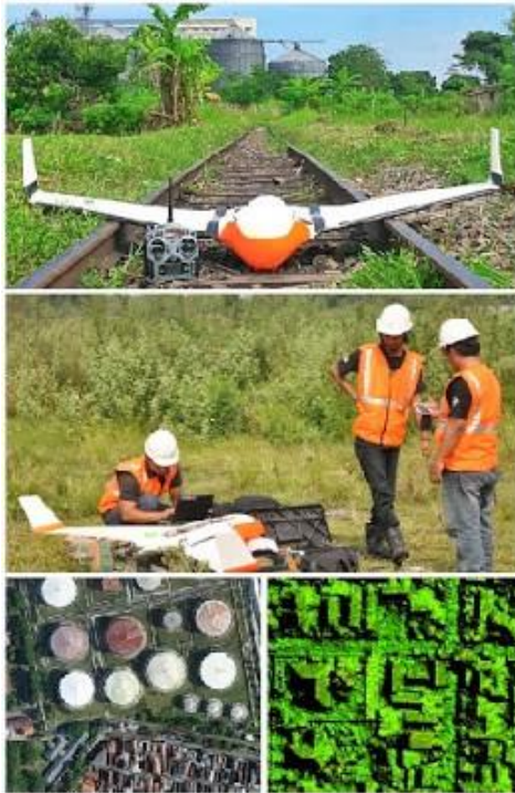
Figure 2 Illustratin of UAV Survey (Jasa Survey Konsultan, 2014)
