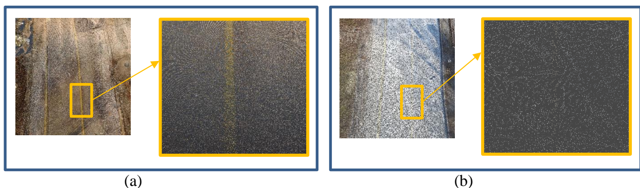
Figure 8. TLS, structured point cloud (a) and UAV, unstructured point cloud (b)
