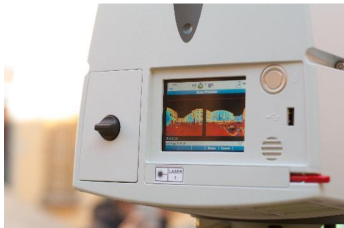
Figura 8 - Leica P30 scanning starting zone "Piazza an Martino"
