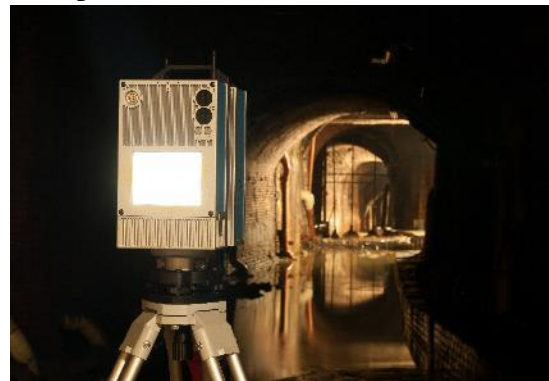
Figura 7 - Z+F 5010x scanning underground
