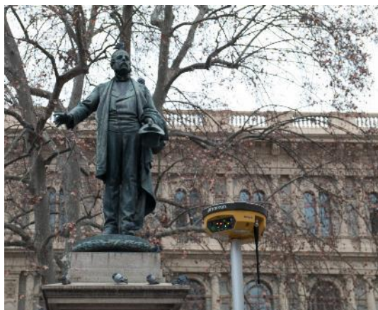
Figura 3 - Georeferencing with static GNSS
