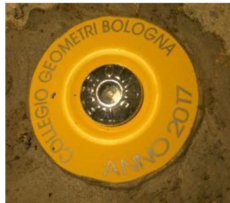
Figura 2 - Permanent survey marker with alloy washer
