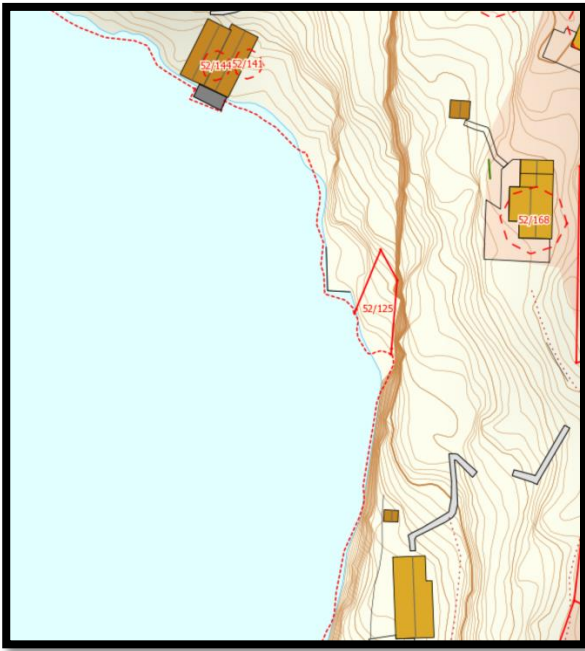
Figure 1: Parcel that is impossible to measure by use of GNSS only.
