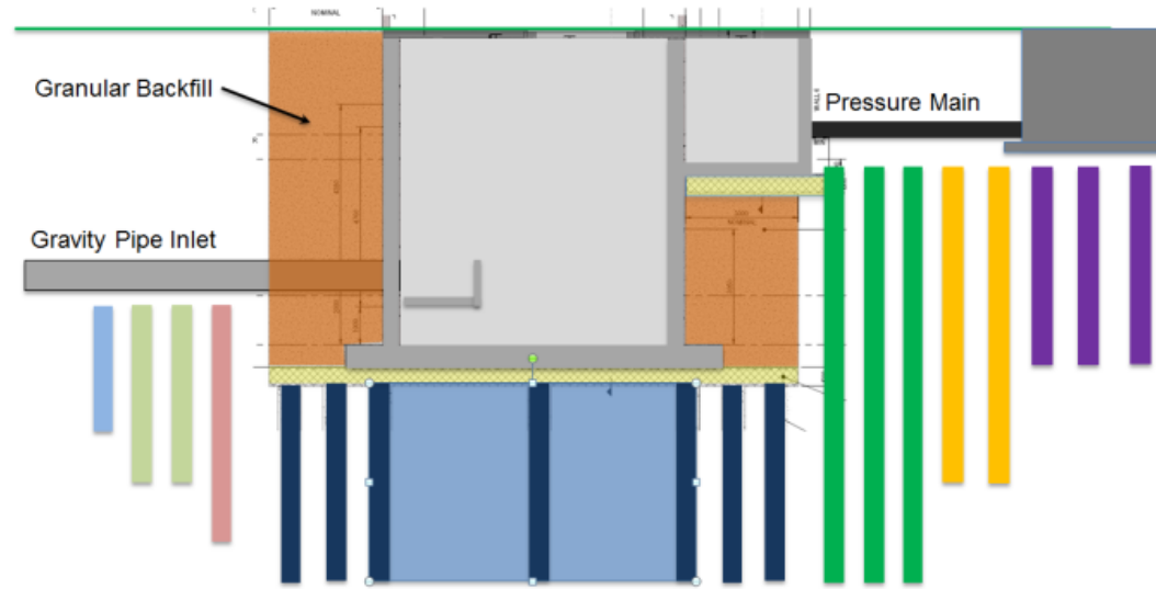
PS136 Typical Cross Section B - B'
