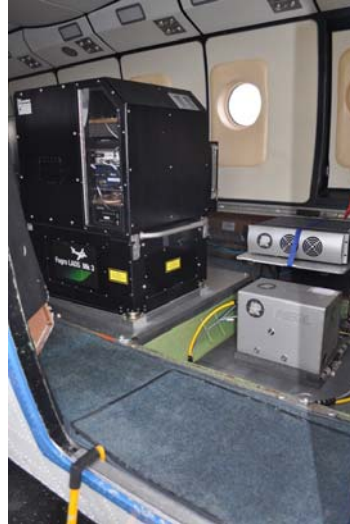
LADS Mk 3 and Riegl VQ820G mounted in CASA 212
