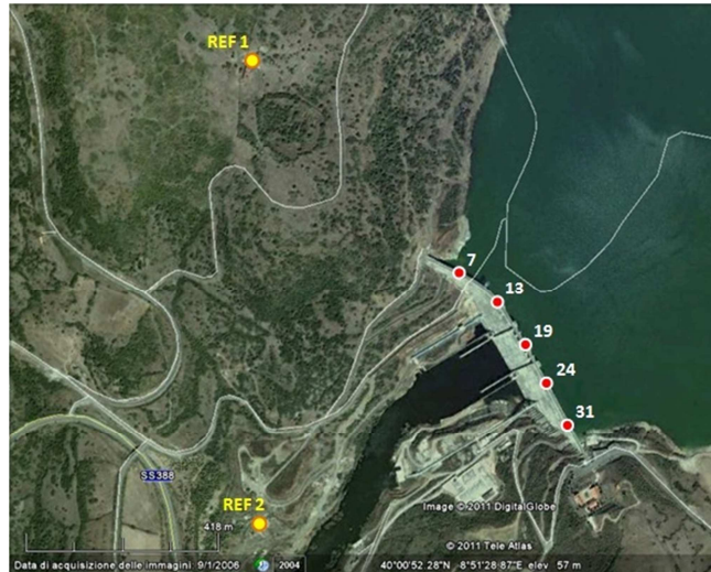
Fig. 12. Cantoniera dam: the planned monitoring GNSS network
