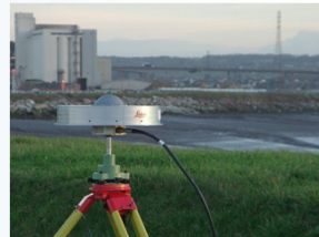
AT504 Choke Ring at One of the Reference Stations at the Avonmouth Harbour
