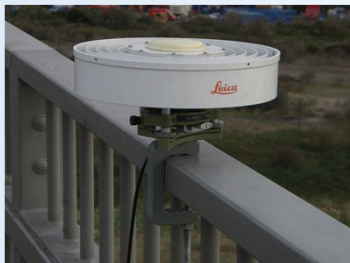
Leica AT503 GPS Antenna Set-up with Clamp and Tribrach Attachment on the Avonmouth Viaduct
