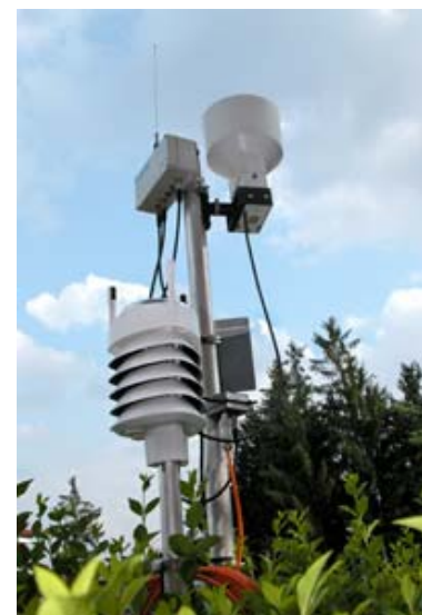
Fig. 4 Sensors system for taking the field data
