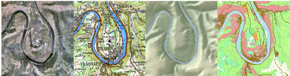
Figure 5 Geospatial basic data countrywide available in Germany, Digital orthophoto (left), topographic map (half left), digital height model (half right), digital landscape model (right)
