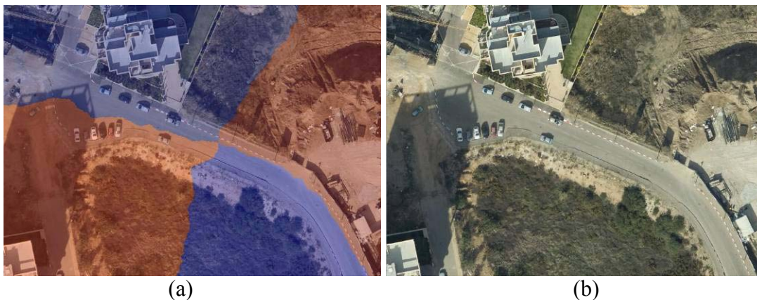
Figure 5. Example of Four images stitched together using the proposed framework. a) Regions taken from different images are marked in different colors. The horizontal seam line runs along the road in order to avoid cutting through the sidewalk, which would cause the seam line to be noticeable. b) The stitching results.
