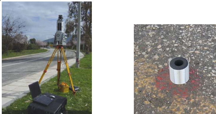
Figure 3: Three set-ups of the scanner were used and registration of scans was performed using retroreflector targets
