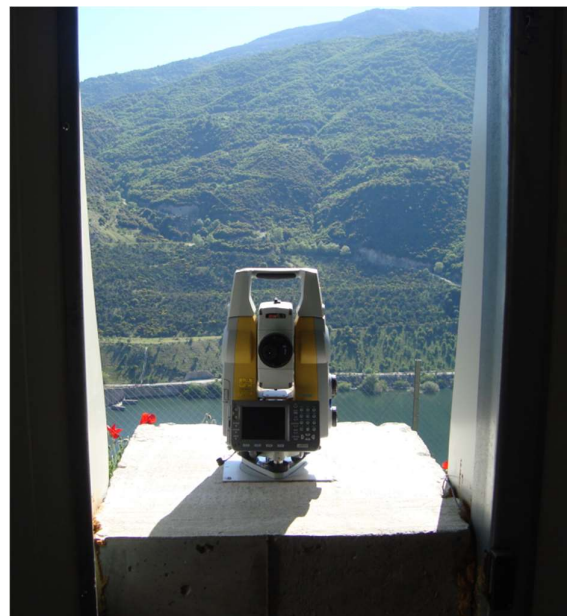
Figure 4. Total Station on left Abutment
