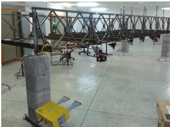
Figure 3. The GBMI system and the 7 CRs at the north side of the bridge.
