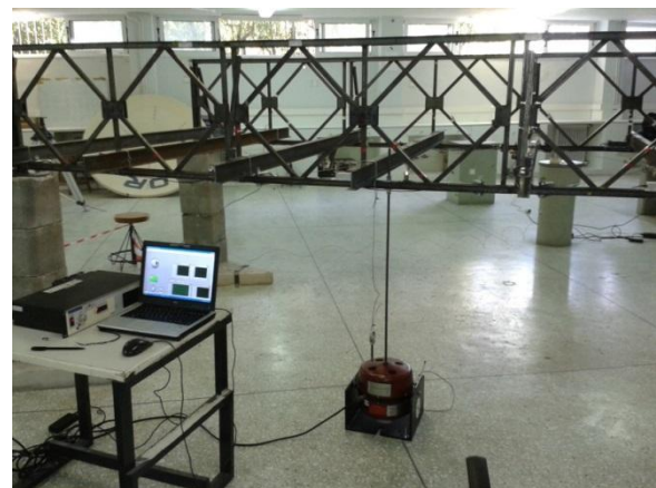
Figure 2: Shaker apparatus setup.
