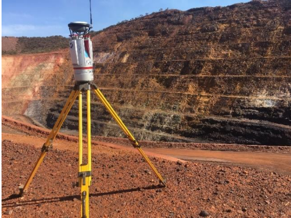
Figure 2. RIEGL laser scanner for surveying an opencast mine (RIEGL, 2019a)
