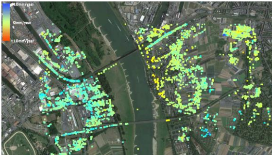
Fig 6 PSI-map for a test area with two bridges over the river Rhine.
