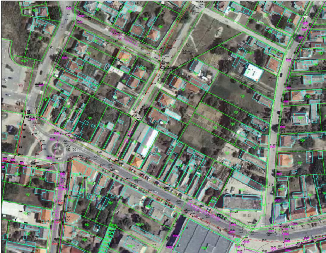
Figure 3. Utility lines on the digital cadastral map – overlapped with digital orthophoto image (town of Beli Manastir)
