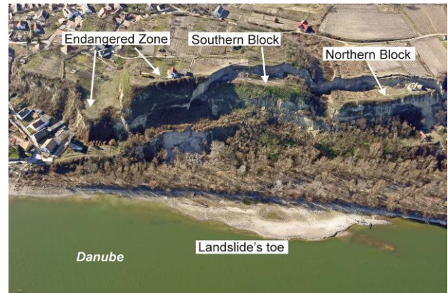
Figure 3. Oblique aerial view of the high bank at Dunaszekcső after landsliding on 12 Feb 2008. The movements spread toward the south in 2010 and 2011 (area indicated by 'Endangered Zone')
