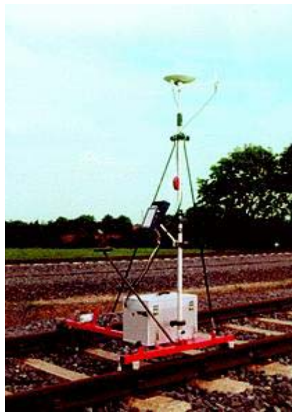
Figure 1: GPS RTK Data Collector-GNBAHN Geo++ ®
