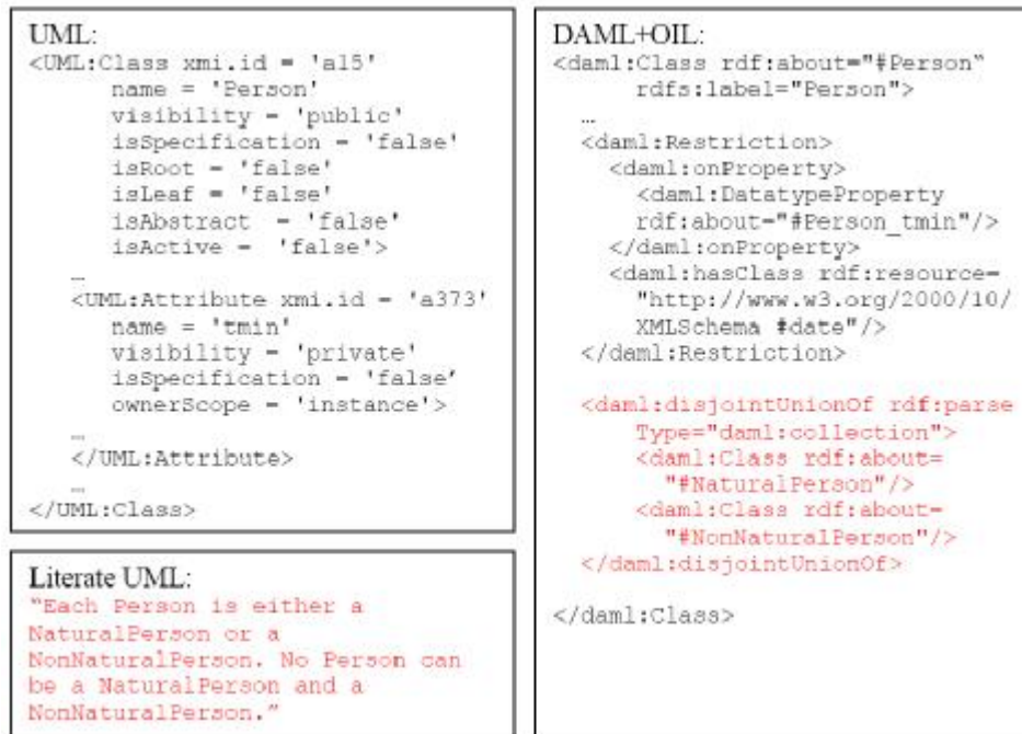
Figure 2 - Transformation UML to DAML+OIL
