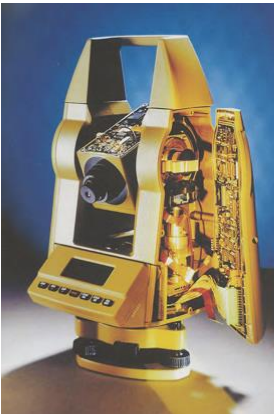
Fig. 6: United: insight into the electronic tachymeter (total station) from 1998 from Heerbrugg with Wild construction design for angle measurement and integrated laser distance meter, based on Einstein's theory (Leica TC500).
