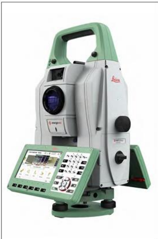
Fig. 13: Multifunctional: the MS60 Multistation from Leica Geosystems Heerbrugg combines Heinrich Wild's theodolite setup with a laser developed from Einstein's theory in two ways: firstly, for distance measurement like a total station and, secondly, with a LaserScan function for capturing, measuring, evaluating and documenting millimetre-accurate 3D laser point clouds.
