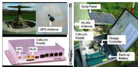
Figure 2, System components of one autonomous station.
