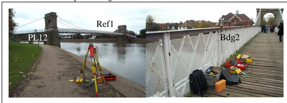
Figure 4: The location of the three pseudolites, with their antennas mounted vertically facing the receiver locations, on the footpaths alongside the River Trent
