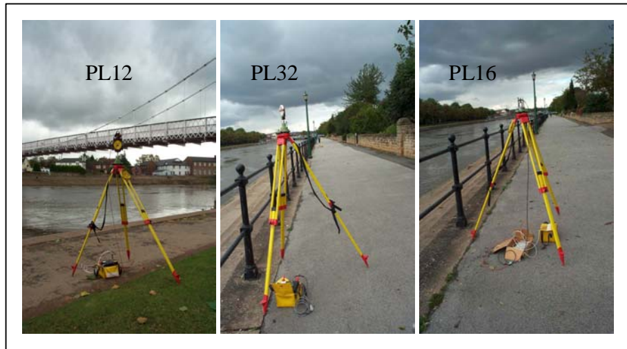
Figure 4: The location of the three pseudolites, with their antennas mounted vertically facing the receiver locations, on the footpaths alongside the River Trent
